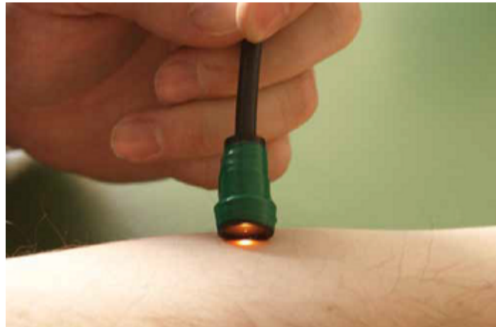
Figure 2: Determination of optical skin parameters and fluorescence with a reflecting measuring head.
