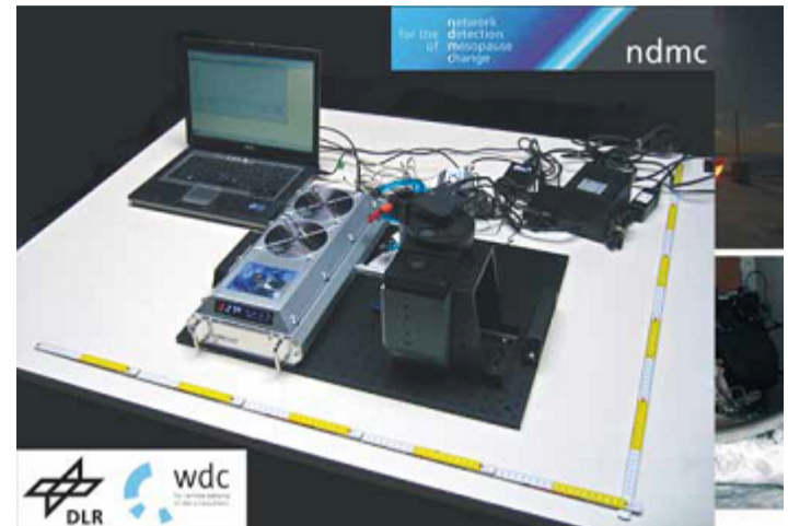
Figure 1: Setup of the GRIPS 6 instrument at the German Remote Sensing Data Center in Oberpfaffenhofen (48.09°N / 11.28°E). The instrument is composed of an Andor Shamrock 163 non-imaging spectrograph, an Andor iDus DU490A-1.7 photodiode array (partly hidden behind the spectrograph and filterwheel), powered by a PS-25 power supply for deep cooling temperatures in combination with an Exos-2 water recirculator. The laptop shows a 15 second exposure of the OH nightglow between 1500 nm and 1600 nm obtained with the Andor Solis software.
