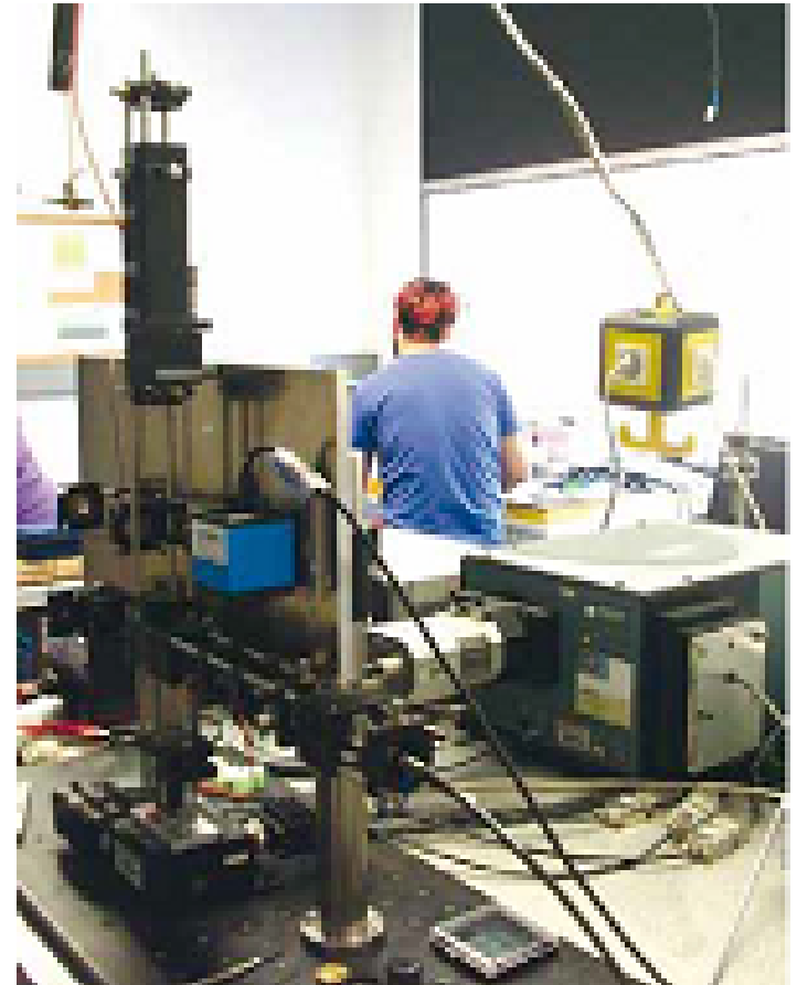
Fig.1a: Experimental setup of the confocal microscopic spectrometer including LED (1), imaging camera (2), motorized stage (3), spectrometer detector combination (4), round-to-angular fiber bundle (5).
