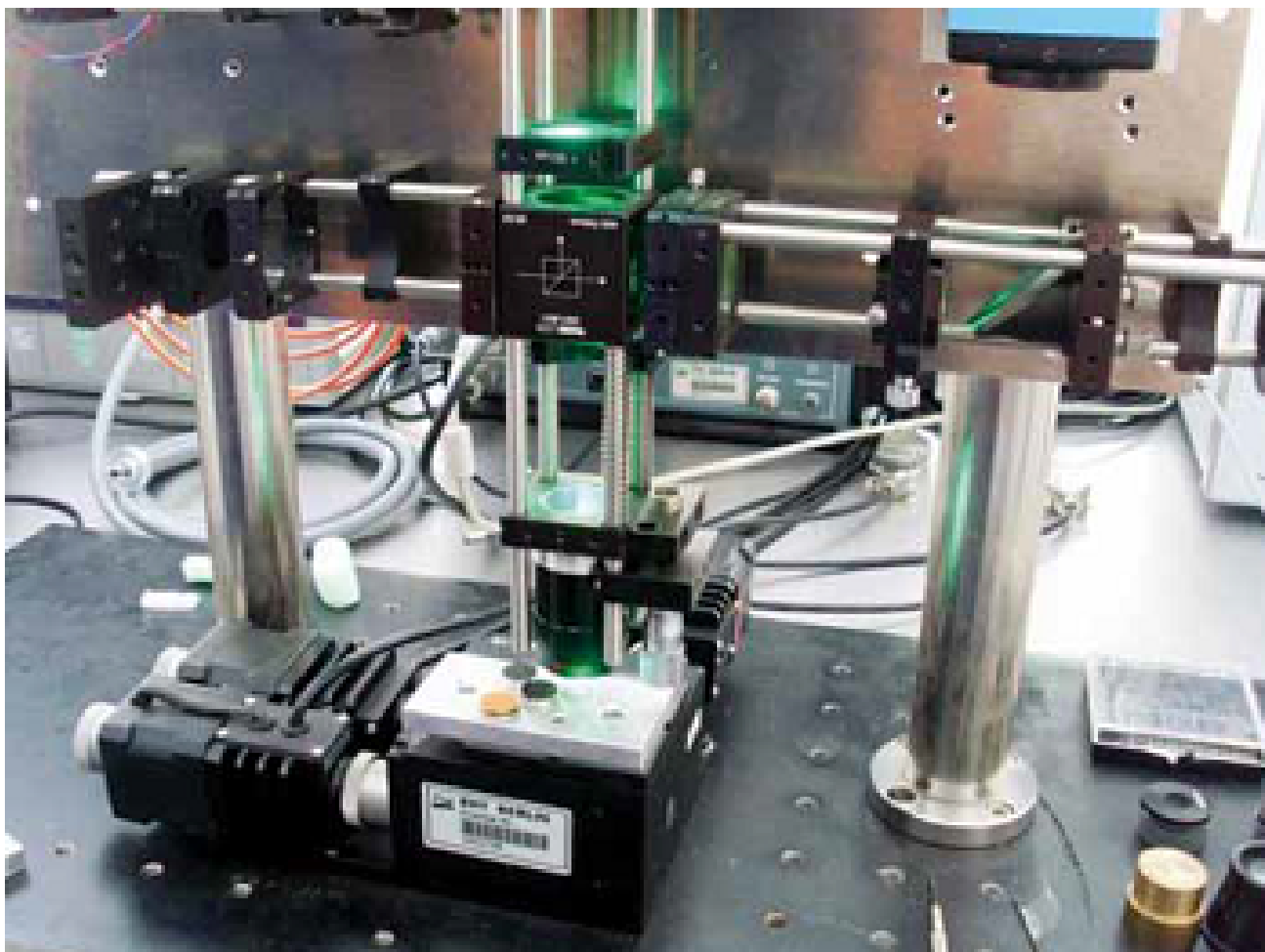
Fig.1b: Detailed image of the objective and the sample holder for correlative SEM microscopy.
