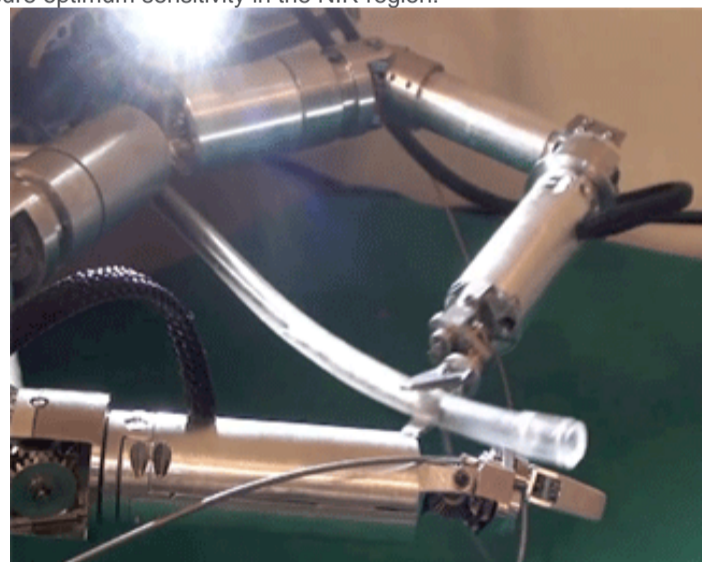
Figure 2: The fiber probe being held and manipulated by the robotic arm of ARAKNES.
