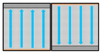
**Figure 2**: LightScan PLUS enables the rolling shutter to scan the sensor from top to bottom or vice versa in one continuous sweep. This is also known as Single Port Readout.
