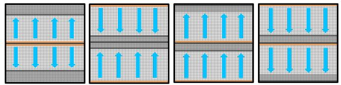
**Figure 3**: Multiple 'dual laser' scanning options available. The standard rolling shutter scan mode (Centre outwards in both directions simultaneously) is illustrated on the left along with the three additional scanning options.
