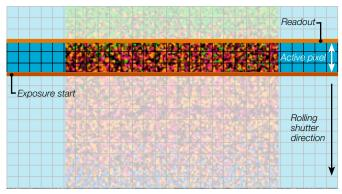
**Figure 1**: Rolling Shutter mode. The highlighted window of pixel rows is exposed to light. This band sweeps from the top to the bottom of the sensor and can be synchronized to the sweep of an illumination laser.
